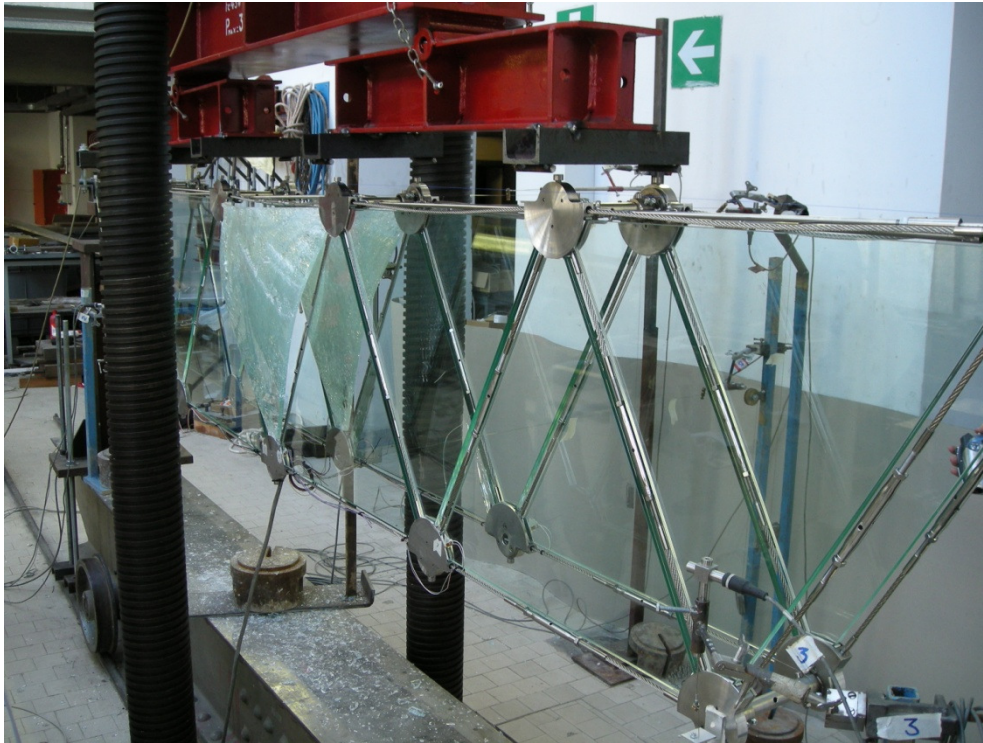
Fig.18 TVT \beta at collapse
